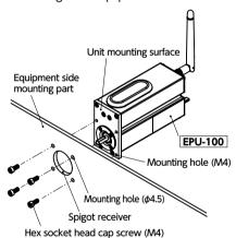
Equipment side mounting part recommended machining dimensions
