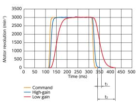
t<sub>1</sub>: Stabilization time at high-gain t<sub>2</sub>: Stabilization time at low-gain
