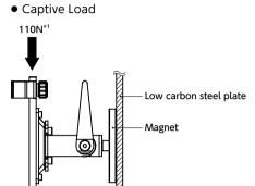
\*1: Captive load is a test value with stable static load. With the magnet securely attached to the material surface of a 10 mm thick low carbon steel plate under room temperature, load was applied from above, and the load at which the magnet separated from the material surface was measured.
