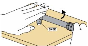
\*1: When the edge does not bite in and slipping occurs, remove SKEK using a socket wrench, and tap it lightly with a plastic hammer until it bites into a hex head bolt, hex nut, etc.
