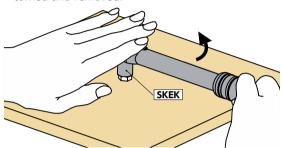
\*1: When the edge does not bite in and slipping occurs, remove **SKEK** using a socket wrench, and tap it lightly with a plastic hammer until it bites into a hex head bolt, hex nut, etc. Hitting with a hammer will transmit the impact to the part where the screw is attached. Be sure to pay attention to the place of use.
