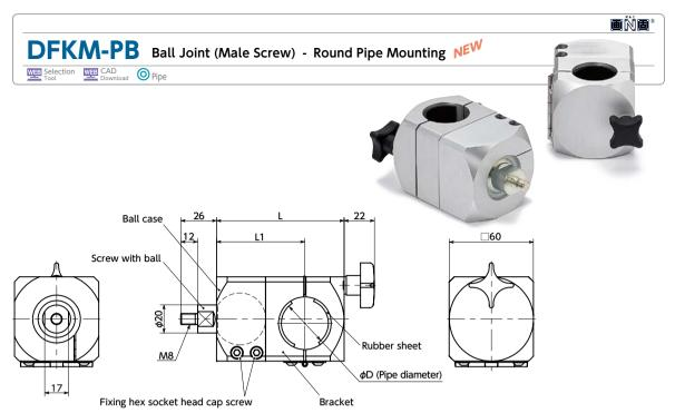
Material/Finish RoHS2 Compliant **DFKM-PB** A6063 Ball Case Anodized S45C Screw with ball Trivalent Chromate Treatment Fixing Hex Socket Head Cap Screw SCM435 (M5×16mm) Ferrosoferric Oxide Film A6063 Bracket Anodized NR (Natural Rubber) Rubber sheet
