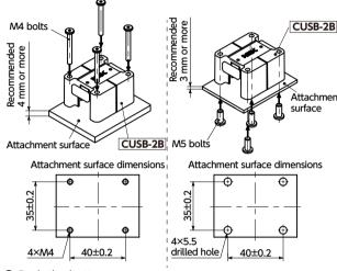
2 Push the button on **CUSB-2B** to release the lock and mount **CUSB-2B** onto the square shaft.
