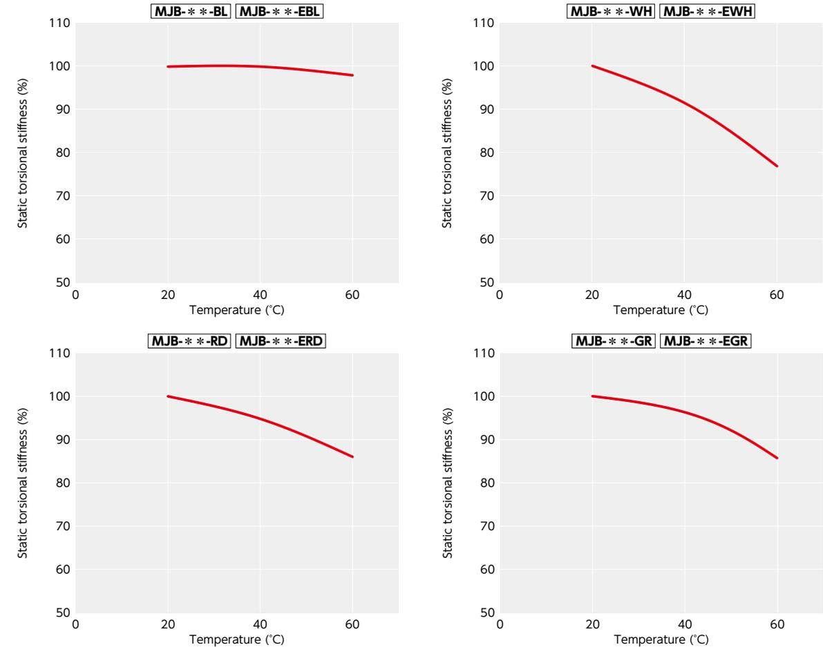
This is a value under the condition where the static torsional stiffness at 20°C is 100%. Changes in the static torsion spring constant within the operating temperature are shown in the graph. Before using the unit, be aware of the deterioration of responsiveness.
