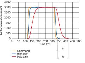
t1: Stabilization time at high-gain t2: Stabilization time at low-gain
