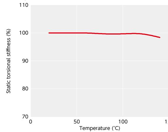
This is a value under the condition where the static torsional stiffness at 20°C is 100%. The change of **XHW-C** and **XHW-AC** in torsional stiffness due to temperature is small and the change in responsiveness is extremely small. If the unit is used under higher temperature, be careful about misalignment due to elongation or deflection of the shaft associated with thermal expansion.
